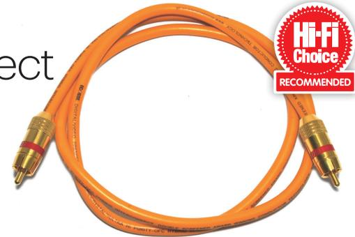
**AS AN ENTRY-LEVEL** digital interconnect, Ecosse's The Producer doesn't shirk its responsibilities to maintain the all-important 75ohm characteristic cable impedance required. This enables it to transmit the pulsed square wave high-frequency signal without internal reflections.
