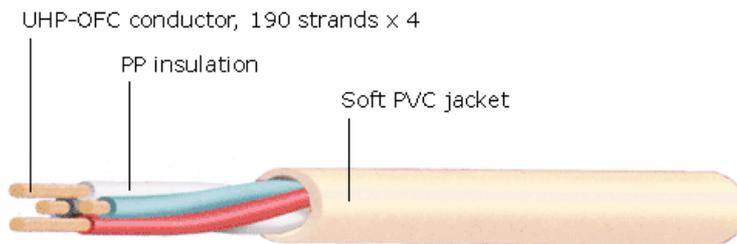
carefully bound in a concentric and tight lay, then twisted. Twisting of the conductors is necessary to overcome the so called 'proximity effect' that naturally occurs when 2 conductors are close to each other and can affect the frequency response of the audio signal, specifically increases at the low frequency (bass) end.
